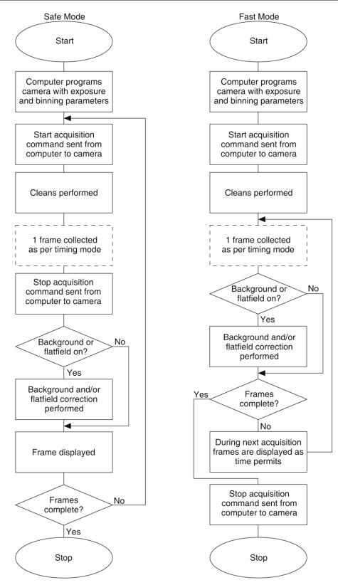
Figure 36. Chart of Safe and Fast Mode Operation
